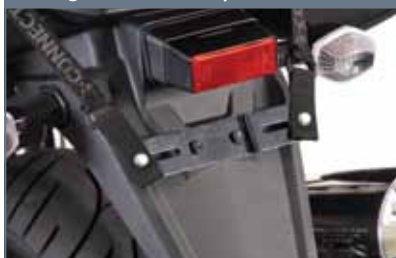
D-Rings bolt to license plate mounts
