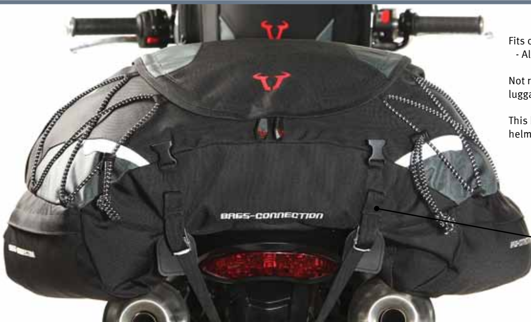
Elastic loops safely stow any excess strap length
