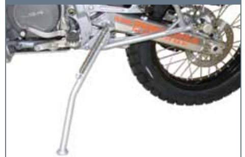
Sidestand with retracted Centerstand
