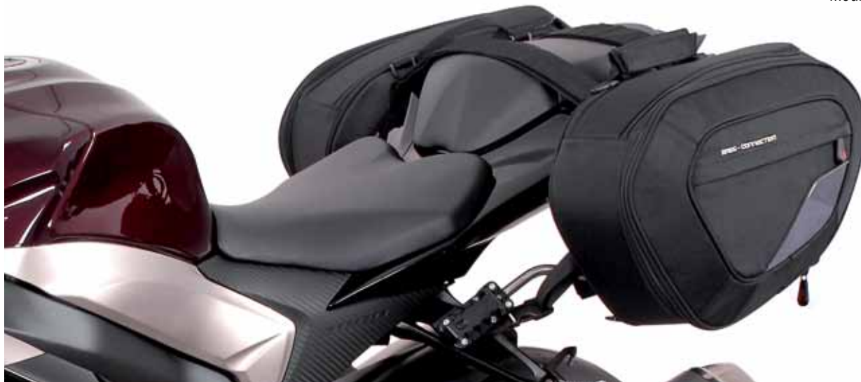
Support Arm Holders bolt on to passenger footpeg mounts
