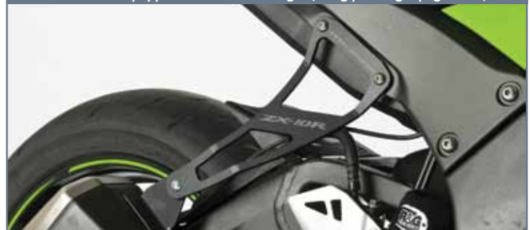
Kawasaki ZX10R equipped with Exhaust Hanger (using passenger peg mount)
