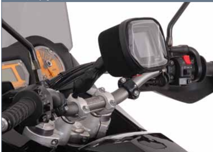
GPS mounted on RAM Mounting System with Bags-Connection Device Pocket (see page 59).
