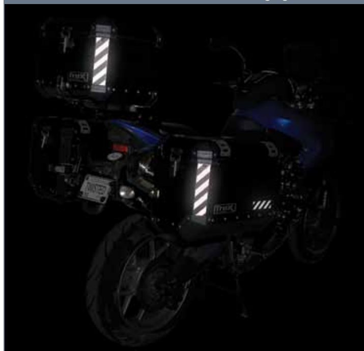
TraX ALU-BOX cases with black ReflectGard kit reflecting high beams.
