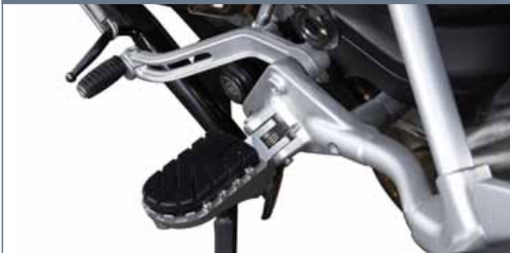
Large teeth provide maximum grip in slippery off road conditions
