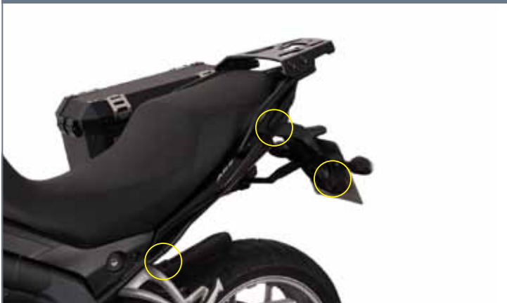
Thumb-sized mounting points remain on the bike when carrier is removed
