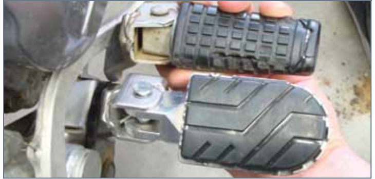
Rubber pad is removable with one bolt
