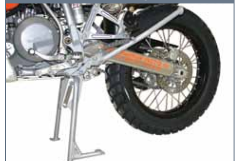
Sidestand with retracted Centerstand
