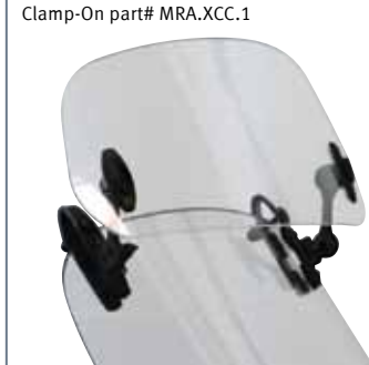
Honda VFR1200F with X-creen Spoiler clamped to the original screen
