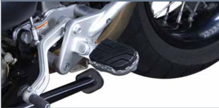
Removable rubber pad reduces vibration during street riding
