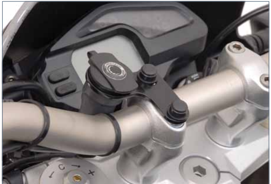
Handlebar mounted for 12-Volt socket.
