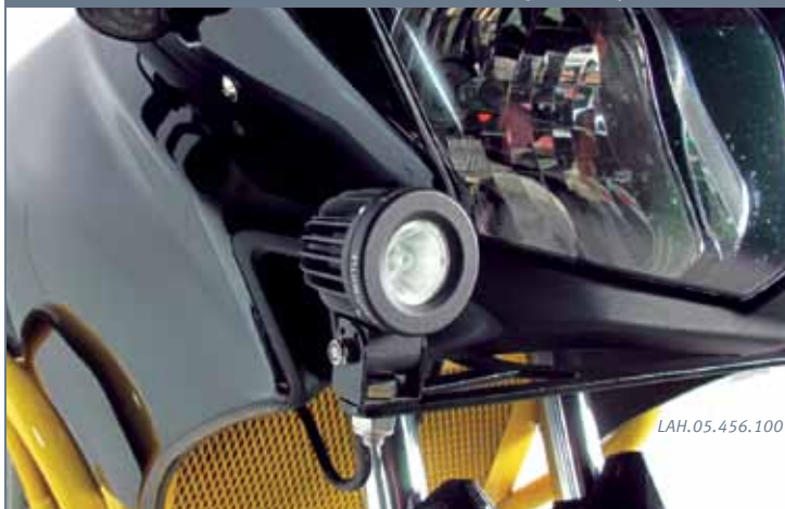
Denali LED lighting mounted on Honda Varadero fairing mount
