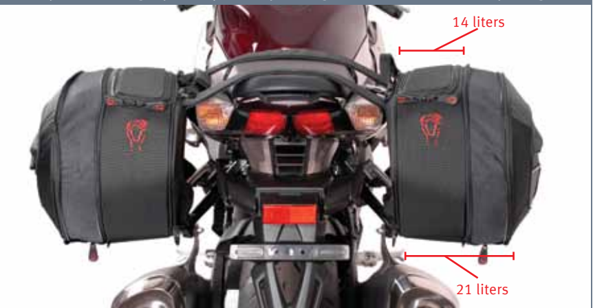
Each Sport Saddlebag expands by 2.75", providing a volume of 14 to 21 liters per bag
