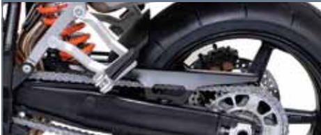
QUICK-LOCK EVO Sidecarrier mounting points
