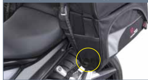
D-rings keep straps from scratching paint
