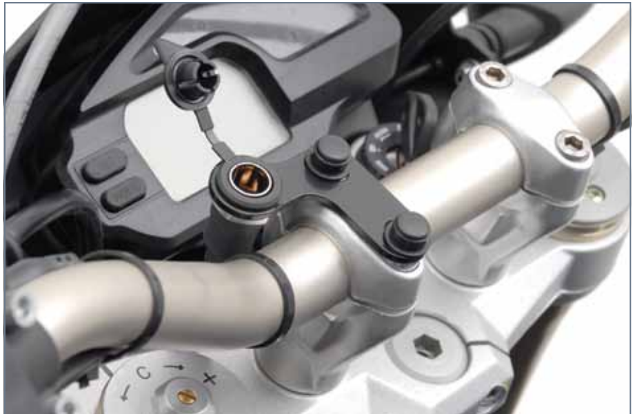
Handlebar mounted 12-Volt Mini-Euro Socket.
